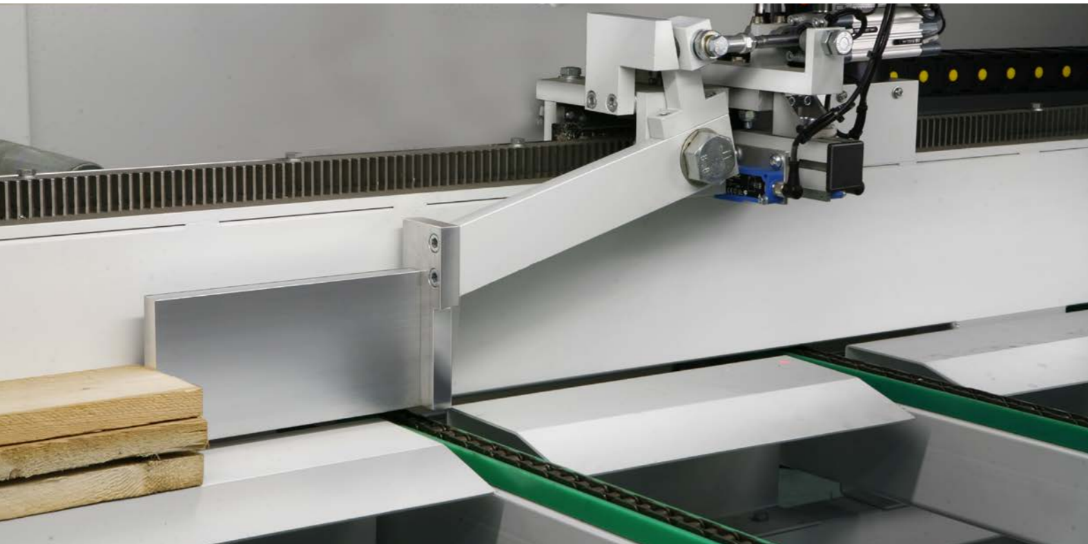
^ Pusher-carriage with top-bottom pneumatic clamp
