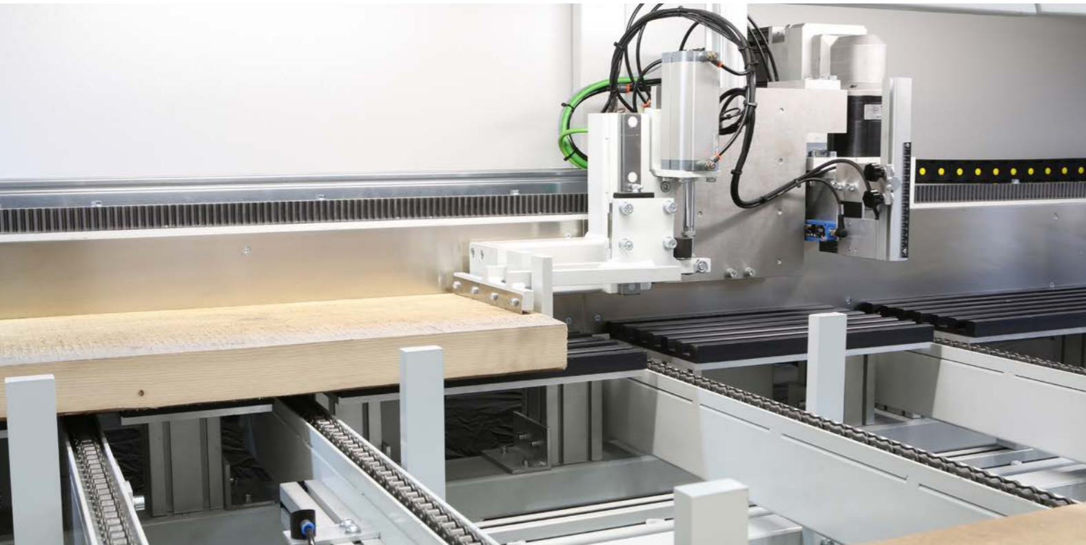
^ Pusher-carriage with top-bottom pneumatic clamp
